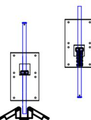
**Keyed Exterior Lock** operates both the Heavy duty Spring Head Bolt and Stainless Steel Foot Bolt for building access through the Hinged Starter Panel. A stranded wire cable connects the head bolt through the inside lock to the foot bolt. Standard operation of the Starter panel causes the large door to open. This can be opened from the inside mounted handle as well. Standard Overhead Door industry Lock is used.
