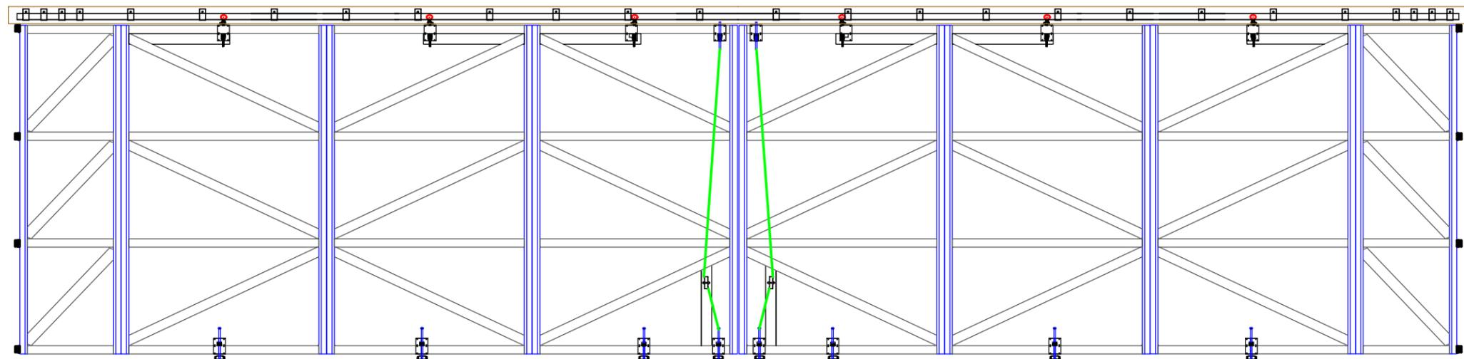
**The Accordion Door Panel** width, inset dimension, quantity of panels and load on the trolley each are evaluated to give the most economical door yet meet strength requirements. There is flexibility in this to either increase or decrease the number of panels for specific needs such as a reduction in the inset dimension.
